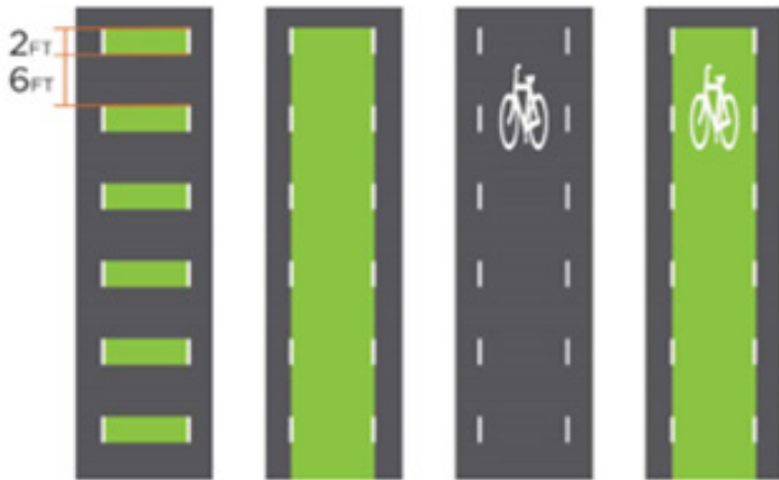
Bike Crossing Markings (Source: Adapted by Kittelson & Associates, Inc. from FHWA Separated Bike Lane Planning and Design Guide)
